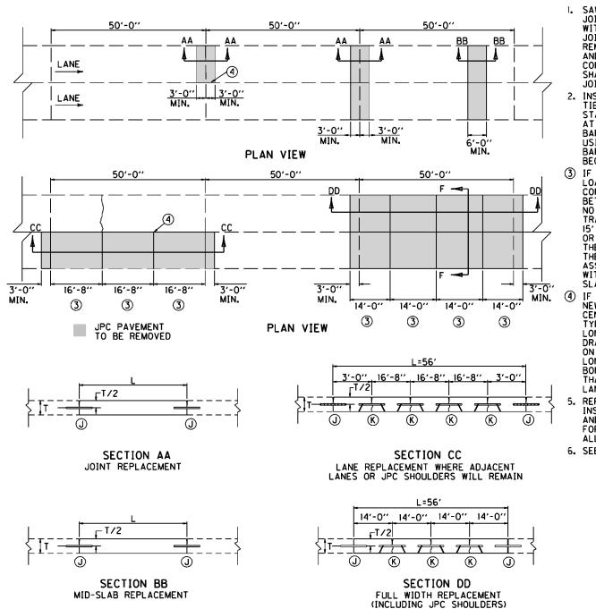
1. SAW AT LOCATIONS "J" AND ALONG LONGITUDINAL JOINT (IF ONLY ONE LANE IS REMOVED) FULL DEPTH WITHOUT DAMAGE TO EXISTING CONCRETE. SAW RELIEF JOINTS AS THE ENGINEER DIRECTS OR APPROVES. REMOVE THE EXISTING JPC PAVEMENT TO THE LENGTH AND AT THE LOCATIONS NOTED ELSEWHERE IN THE CONTRACT. L=6 FEET MINIMUM AND LOCATIONS "J" SHALL NOT BE CLOSER THAN 6 FEET TO ANY TRANSVERSE JOINT BEYOND THE REPAIR.
