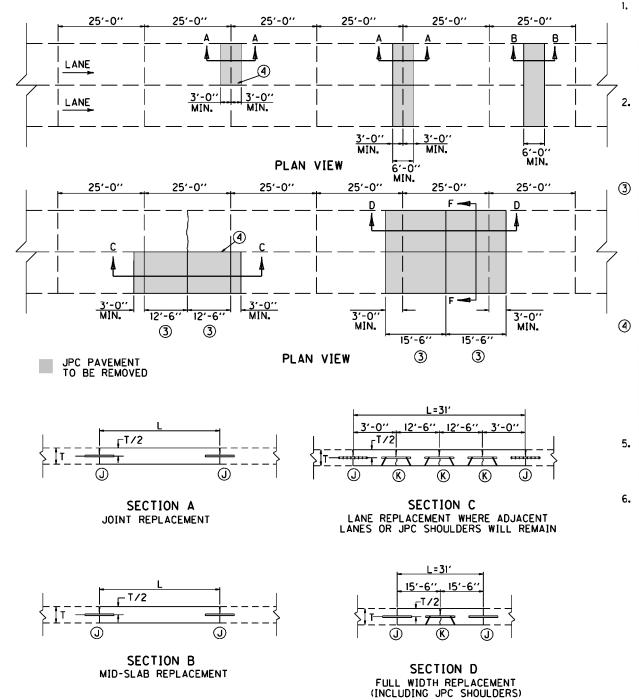
SAW AT LOCATIONS "J" AND ALONG LONGITUDINAL JOINT (IF ONLY ONE LANE IS REMOVED) FULL DEPTH WITHOUT DAMAGE TO EXISTING CONCRETE. SAW RELIEF JOINTS AS THE ENGINEER DIRECTS OR APPROVES. REMOVE THE EXISTING JPC PAVEMENT TO THE LENGTH AND AT THE LOCATIONS NOTED ELSEWHERE IN THE CONTRACT. L=6 FEET MINIMUM AND LOCATIONS "J" SHALL NOT BE CLOSER THAN 6 FEET TO ANY TRANSVERSE JOINT BEYOND THE REPAIR.
